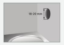
Insert the faucet base through the wall and fix it firmly on the opposite side with the hexagonal nut and the disk.
